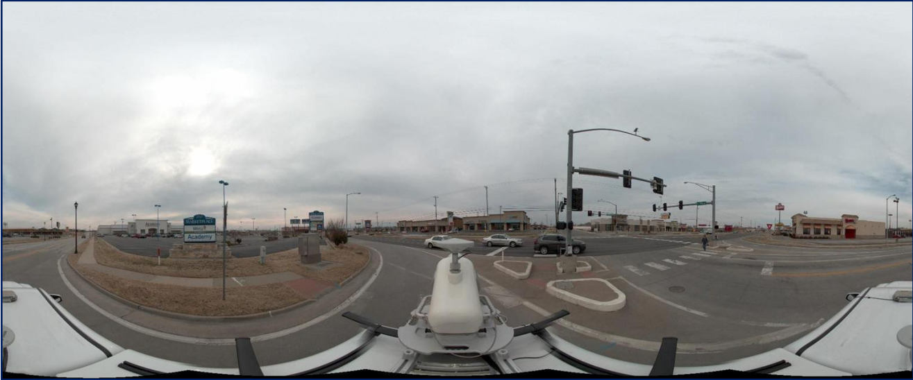
High-resolution spherical output from Ladybug5+ camera displayed in 2D.
