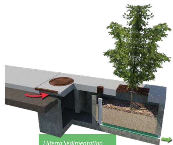
Filterra Sedimentation Chamber (Maryland Only)
