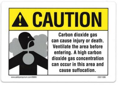
NOTE: Additional signage may be required in accordance with gas detection system's manufacturer specifications.
