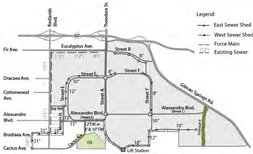
Exhibit 3-20 Wastewater Service Plan
